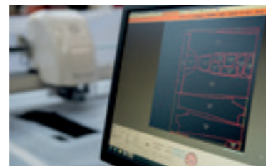
Tool ISO Editor image position, notches, drill holes, lines.
